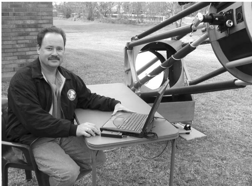
Fig. 1.5 Glenn Schaeffer from Houston, Texas, uses a typical webcam planetary imaging setup. He couples a Philips ToUcam Pro II 840K to his 20-inch Obsession Dobsonian mounted on an Osypowski dual-axis equatorial platform to image the Moon and planets from his backyard. Photo by Glenn Schaeffer.
