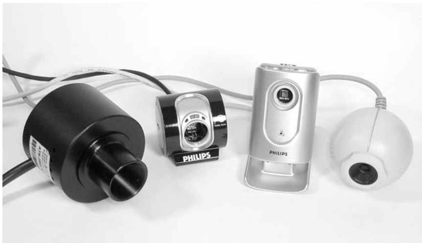
Fig. 1.4 The astronomical webcam “family tree” is shown above. At the right is the original spherical Connectix black-and-white Quickcam that started the long-exposure webcam astrophotography revolution. The Philips ToUcam Pro II that matured webcam astrophotography is next followed by the new generation Philips SPC900NC. At the left is the Atik ATK-2HS, a commercially-modified air-cooled long exposure-capable version of the ToUcam that has allowed the novice to achieve CCD-quality electronic astrophotography. Photo by Robert Reeves.
