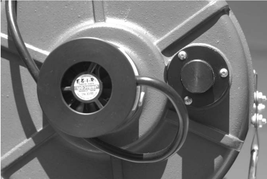
Fig. 1.6 It is easier to view images when the camera's display shows north at the top. When installing the camera, orient it so the display is properly aligned to begin with. With an ATK-2HS on a Celestron-8, aligning the camera cable with the telescope focus knob aligns north at the top of the field. Photo by Robert Reeves.
