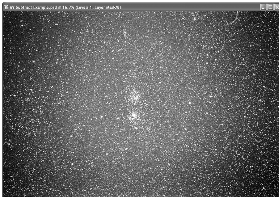
Fig. 6.1 Vignetting from light falloff is clearly evident in this film image of the Double Cluster made by the author. The image was highly stretched to clearly illustrate the problem.
